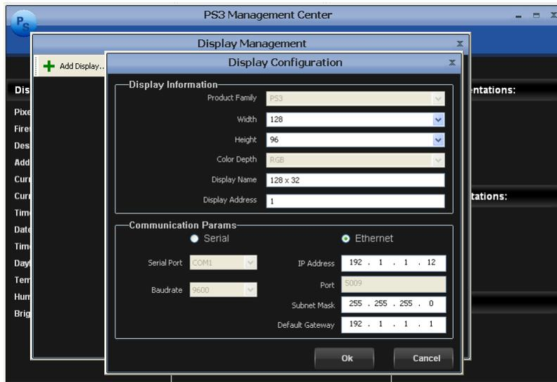
In this step, we can add The size, Display Address, If the sign is connected Serial or Ethernet.
